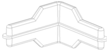
F- Post Inserts (4-ea.) (Used on Storage Rack)
